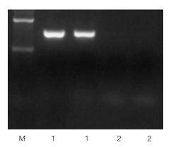
**TEMPase is inactive at ambient temperature**Ampliqon TEMPase is activated by initial heating at 95 °C for 15 minutes (lane 1). Without activation the enzyme is completely inactive (lane 2). M: Marker.
