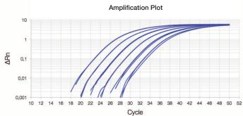
Amplification plot of a fourfold dilution series for Pthr target (75 bp) amplified from human gDNA. Starting amounts of 80 ng gDNA was amplified in triplicates using RealQ Plus 2x Master Mix for Probe with high ROX<sup>TM</sup>.
