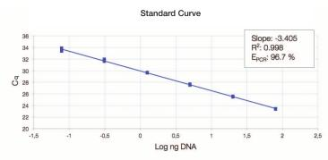
Standard curve based on the adjacent amplification data. This confirms a high linear range, high efficiency and low replicate deviations.
