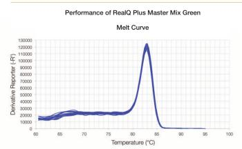
The melt curve analysis detected no non-specific products, which confirm the specificity of the mix.
