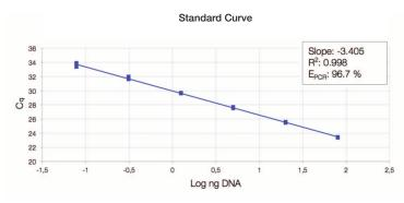
Standard curve based on the amplification data above. This confirms a high linear range, high efficiency and low replicate deviations.
