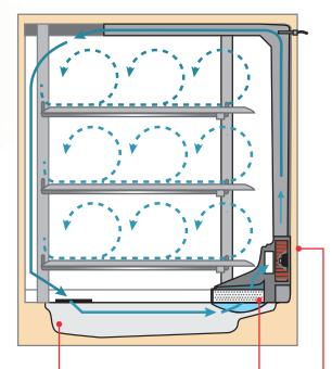
Incoming air first travels over a direct heated water reservoir resulting in 50% faster humidity recovery than with a standard water pan design.\*\*
